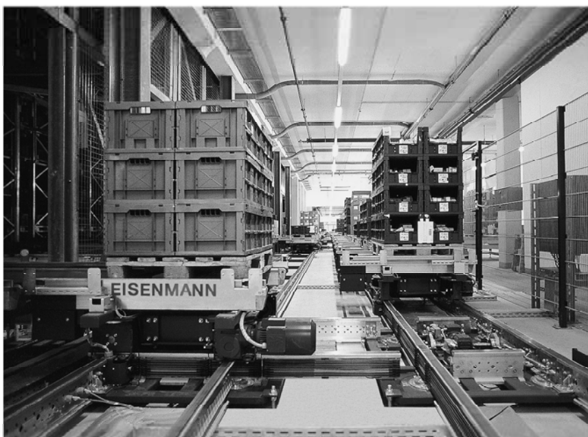
Insulated conductor U 10 in an automated warehouse, woolworth.
