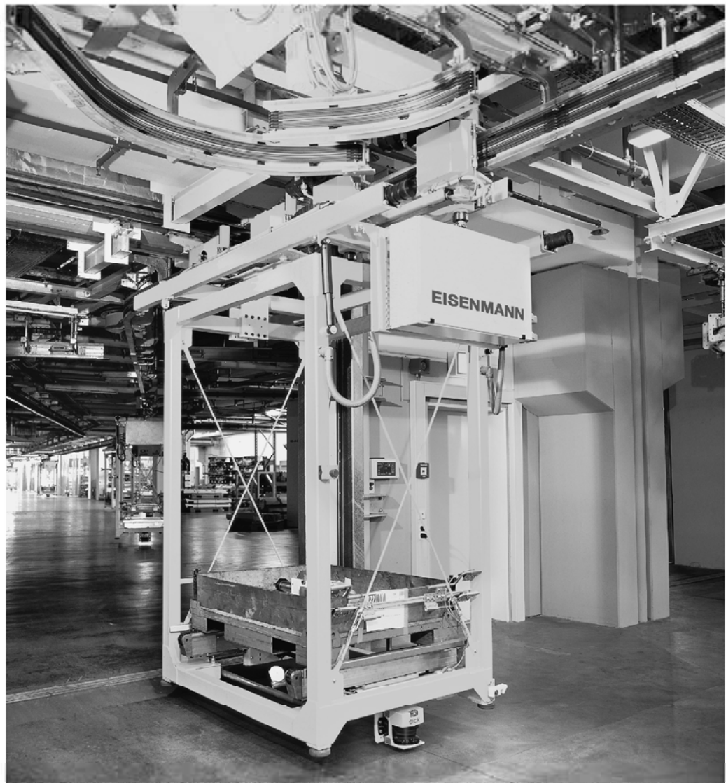
Insulated conductor U 10 in an automated warehouse, woolworth.
